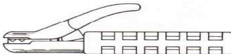
Fig b. Electrode Holder
